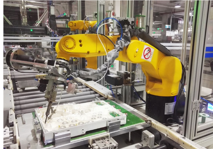
电子元器件锡焊 Tin soldering of the electronic components
