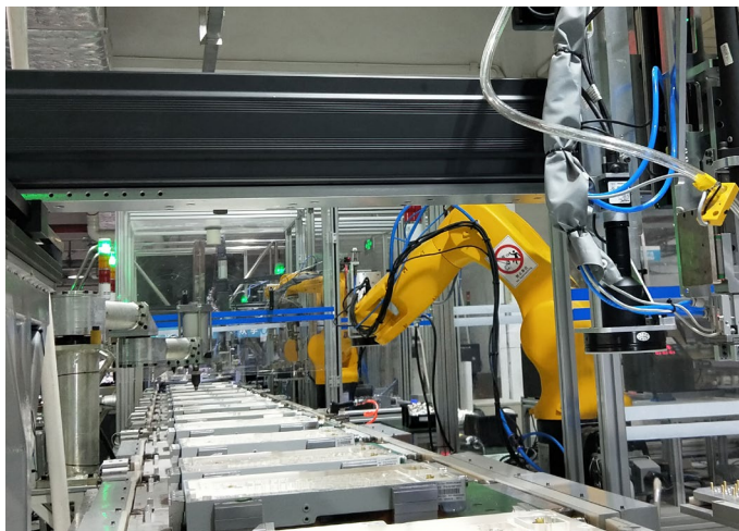
滤波器谐振杆装配，螺丝锁付 Assembly of filter resonant rod , screw lock
