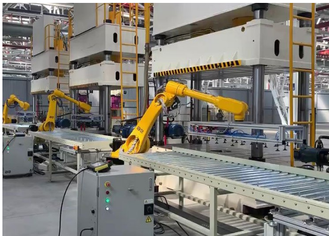
冲压机上下料产线 Press machine loading and unloading production line
