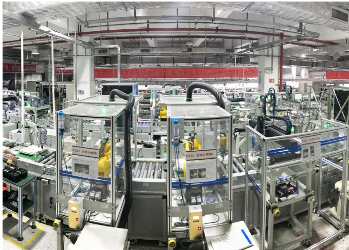
无源滤波器自动化智能柔性装配生产线 Passive filter automatic intelligent flexible assembly line
