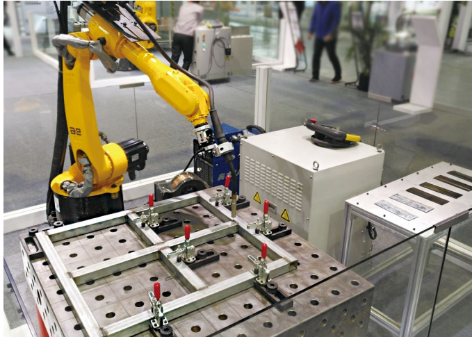
农用机械零部件气体保护焊接 Gas protection welding of the agricultural mechanics components
