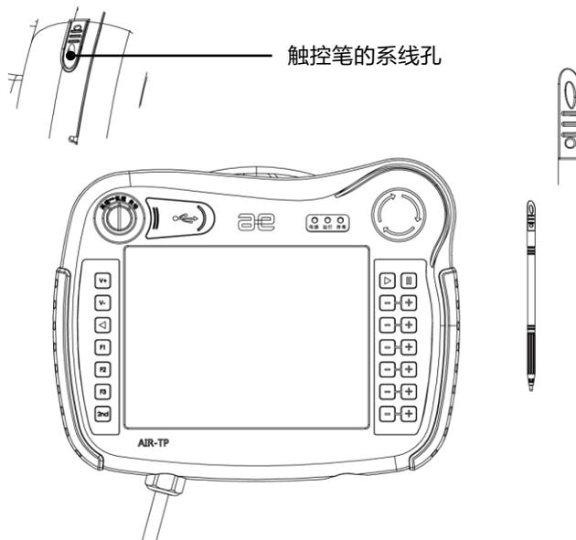
图 2-14 AIR-TP 示教器触控笔
