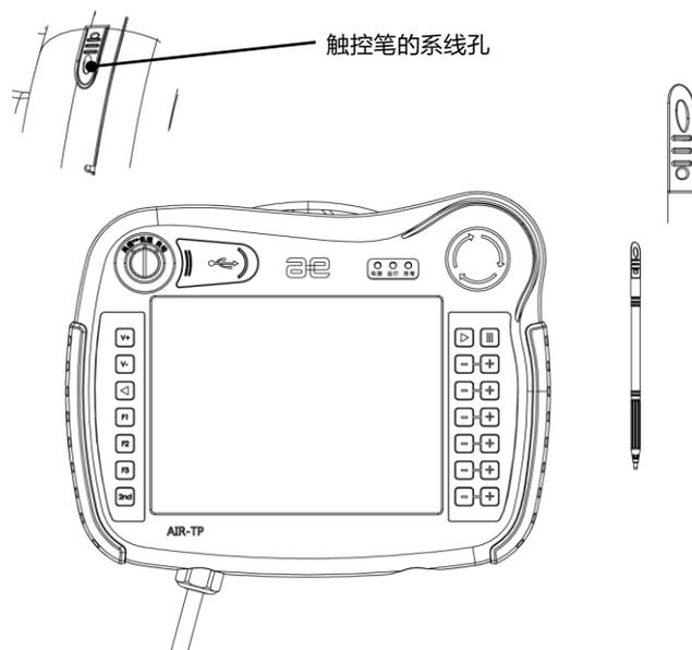
图 2-14 AIR-TP 示教器触控笔
